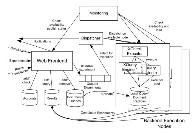
Figure 2. Benchmarking Service Architecture
