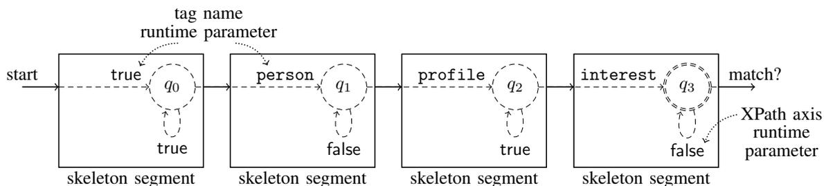
Fig. 3. Two-part “skeleton automaton” design for hardware-based XML projection in *MXQuery/H*. The FPGA configuration mechanisms are used to realize the *static part* of the automaton (drawn as solid lines), whereas all query-specific behavior is covered by the *dynamic part* (dashed lines) that can be parameterized at runtime.
