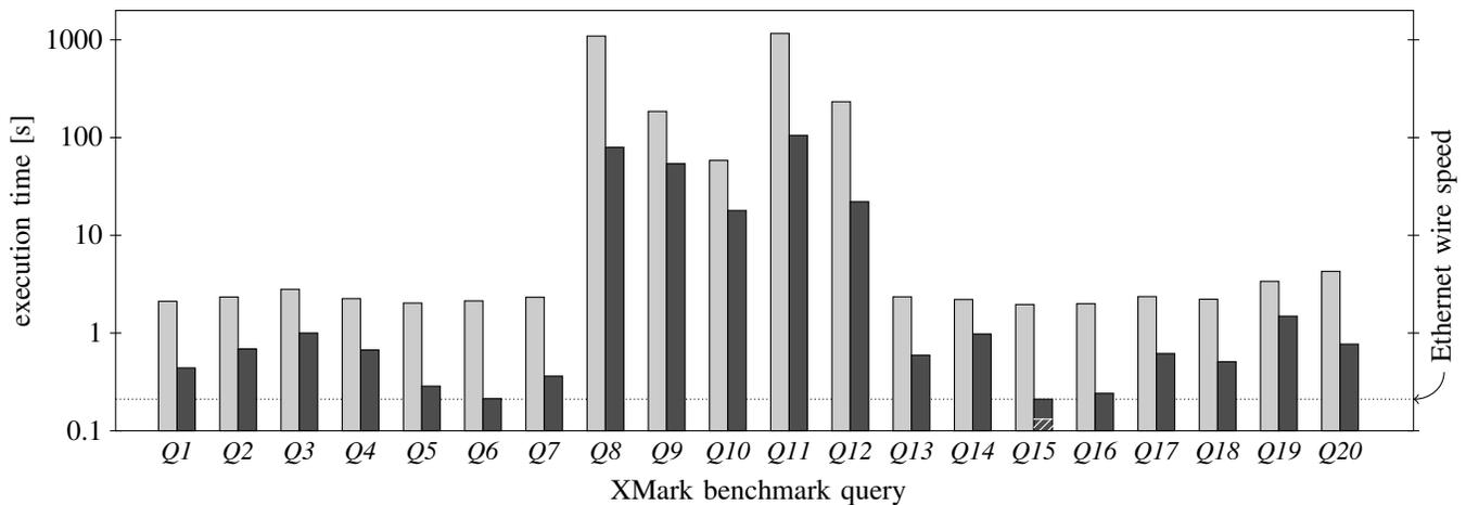
Fig. 5. MXQuery execution times for the 20 XMark queries (scale factor 0.2;  $\approx 24$  MB) before (□) and after (■) input projection. With projection, Query Q15 becomes bound by the physical network speed. Without this bound, Q15 could run significantly faster, as indicated with ▨.
